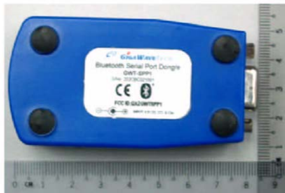
Rear View of the GIGAWAVETECH Bluetooth Serial Port Dongle.
