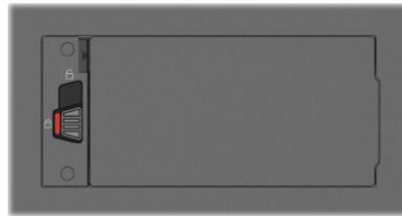
Incorrect (revealing red part)
