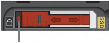
Incorrect (revealing the red part)
