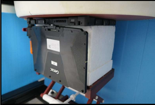
Bottom of EUT Tested at 0 mm
