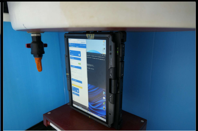
Right Side of EUT with Bat2 Tested at 0 mm
