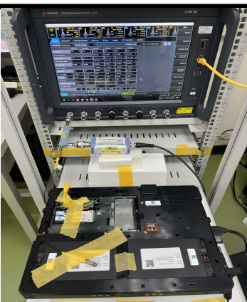
Setup for Conducted Power Test (for 5GNR SA)
