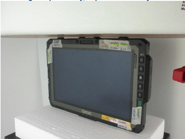
Testing Setup for Body, Top Side w/ Battery at 0 mm
