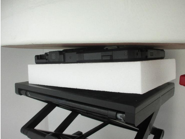
Testing Setup for Body, Bottom Surface w/ Battery at 0 mm
