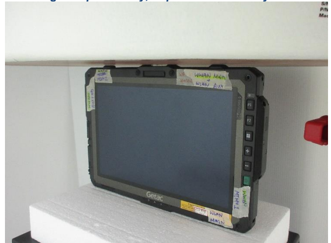
Testing Setup for Body, Top Side w/o Battery at 0 mm
