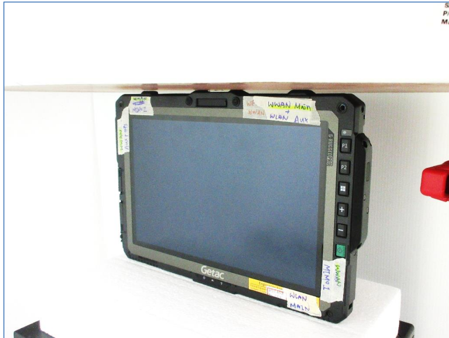
Setup for SAR Testing (Body, Tablet mode, Top Side at 0 mm)
