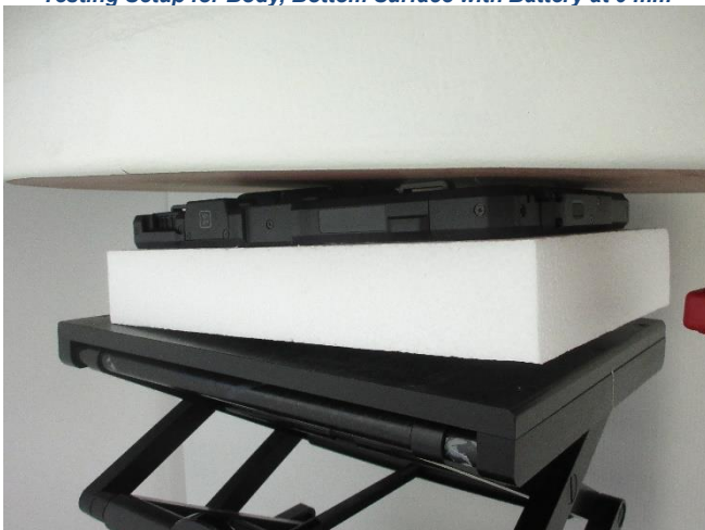
Testing Setup for Body, Bottom Surface with Battery at 0 mm
