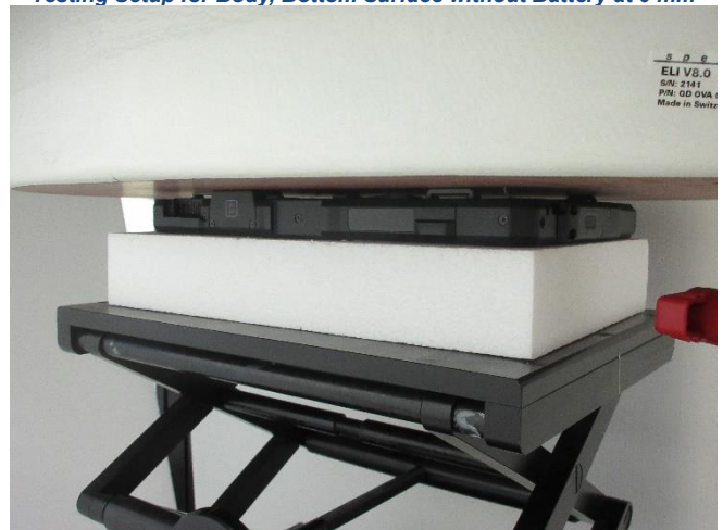
Testing Setup for Body, Bottom Surface without Battery at 0 mm
