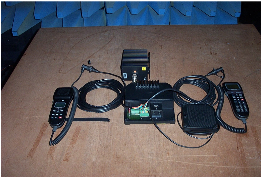
PHOTOGRAPH 2 Close up view of RS81/2 during radiated emissions testing
