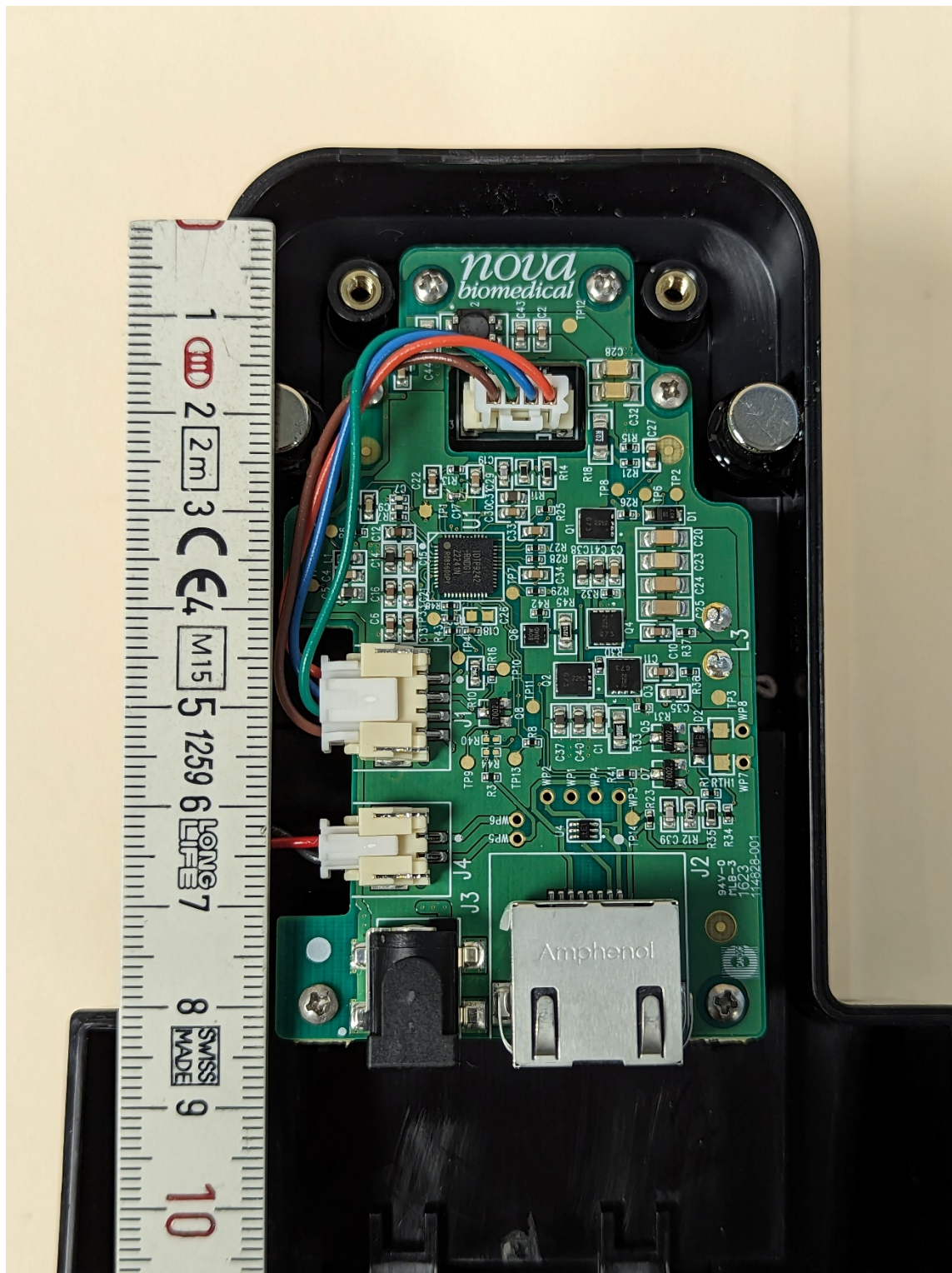
Main PCB in enclosure
