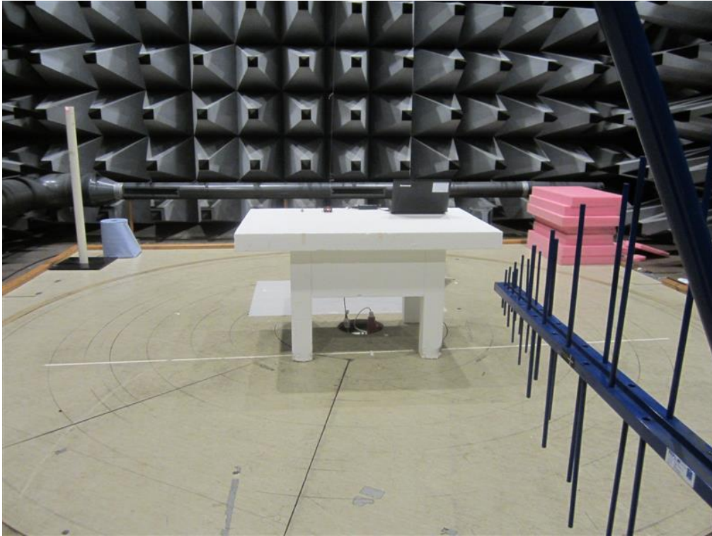
Photo 4.5.1 Test setup regarding measurement of radiated emission (below 1 GHz).
