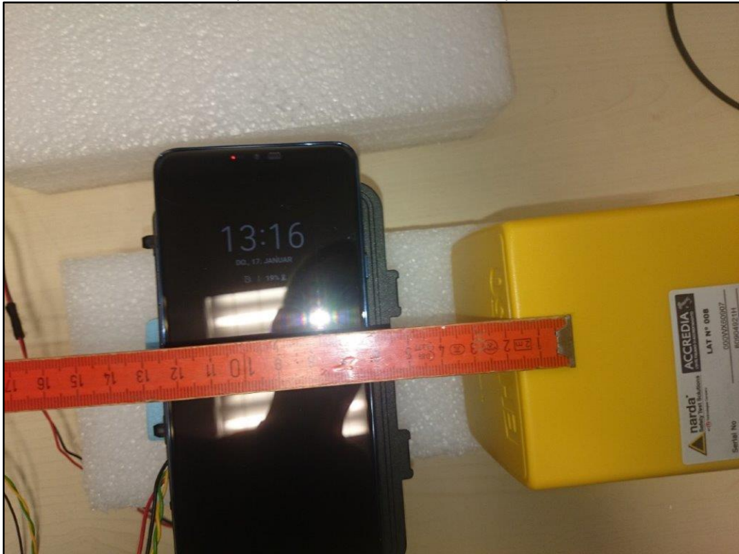
Photo 18: Test position – top side – Wireless charging with EHP50F probe (Samsung Galaxy Note9 / 5cm distance)
