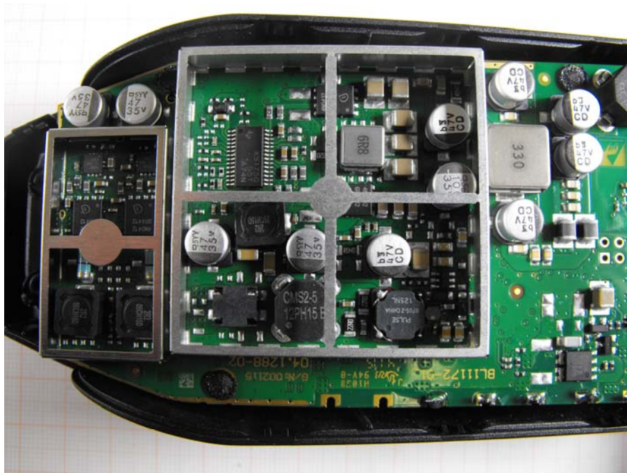
Photo 2: Main board, shielding removed
