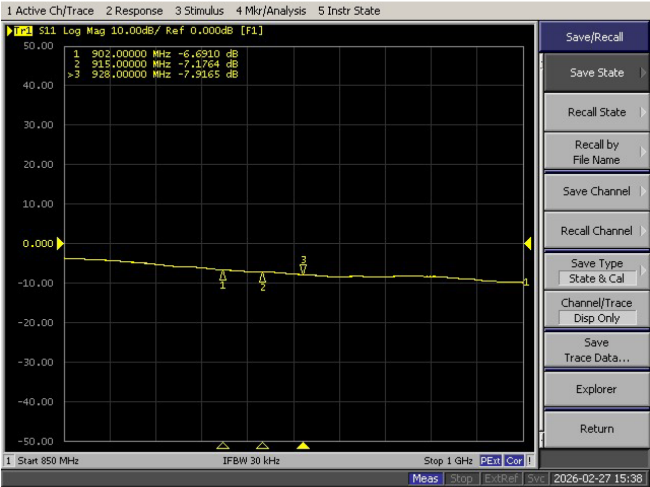
Figure 13: Antenna return loss
