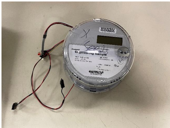
Figure 1.4.1-3 –Front view of the host meter
