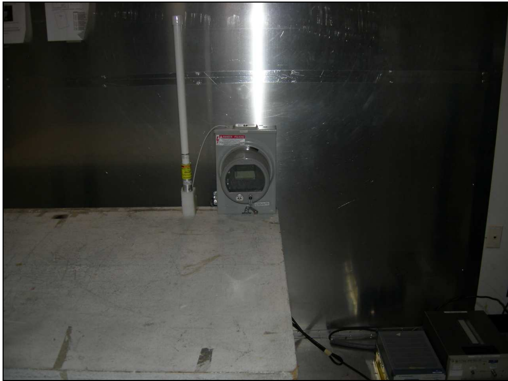
Figure 9: Conducted Emissions – Monopole Antenna
