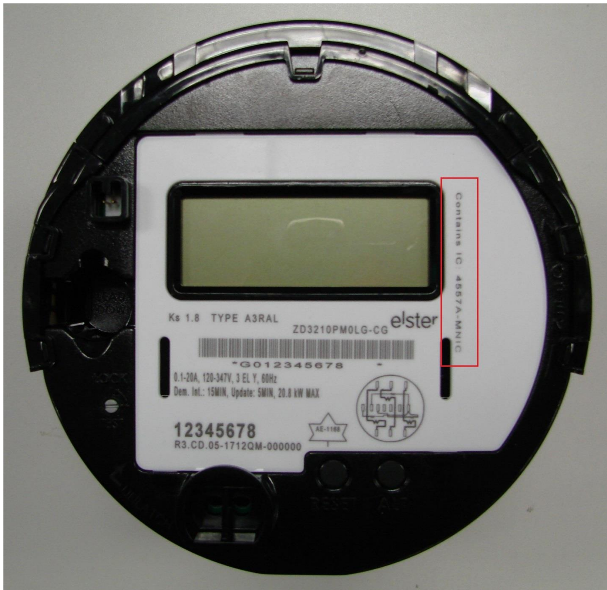
A3 electricity meter front view, showing IC: 4557A-MNIC
