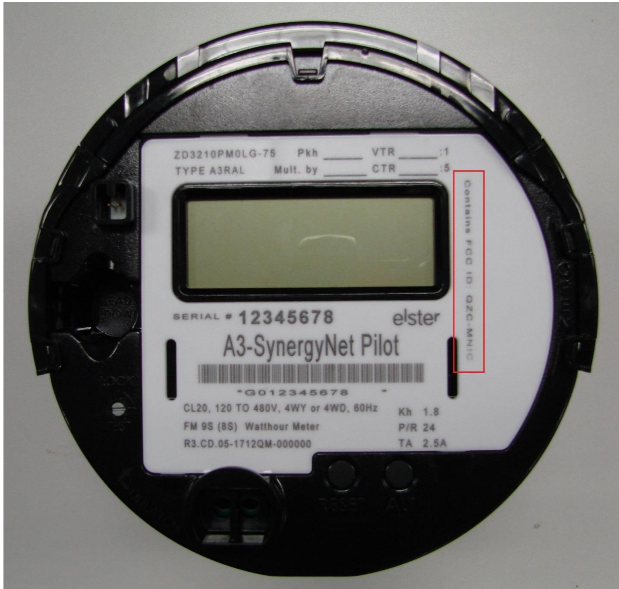
A3 electricity meter front view, showing FCC ID: QZC-MNIC
