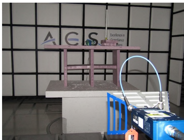
Figure 5: Radiated Emissions – Above 1 GHz (Half-Wave Dipole Antenna) – Front View
