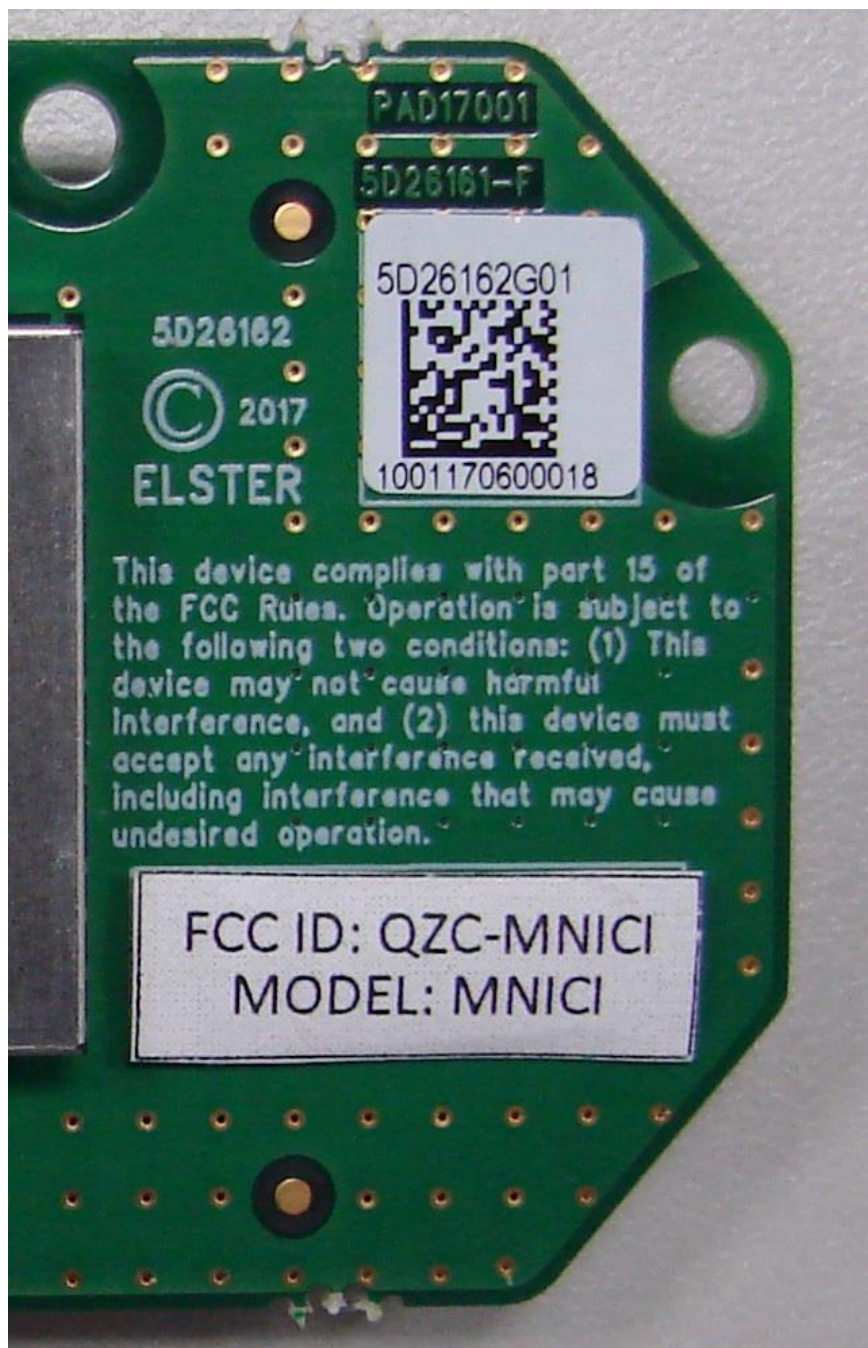
MNIC PCBA top view, showing FCC ID detail
