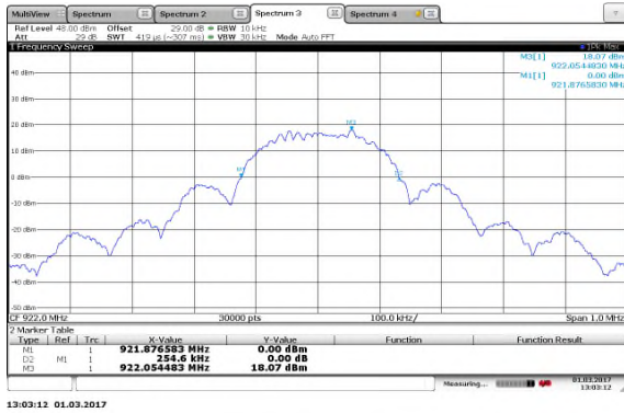
Figure 7.4.4.2-8: 20dB BW Mid Channel 200kbps
