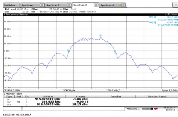
Figure 7.4.4.2-7: 20dB BW Low Channel 200kbps
