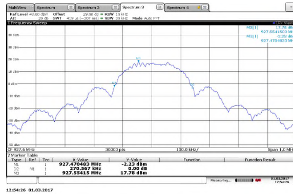
Figure 7.4.4.2-9: 20dB BW High Channel 200kbps
