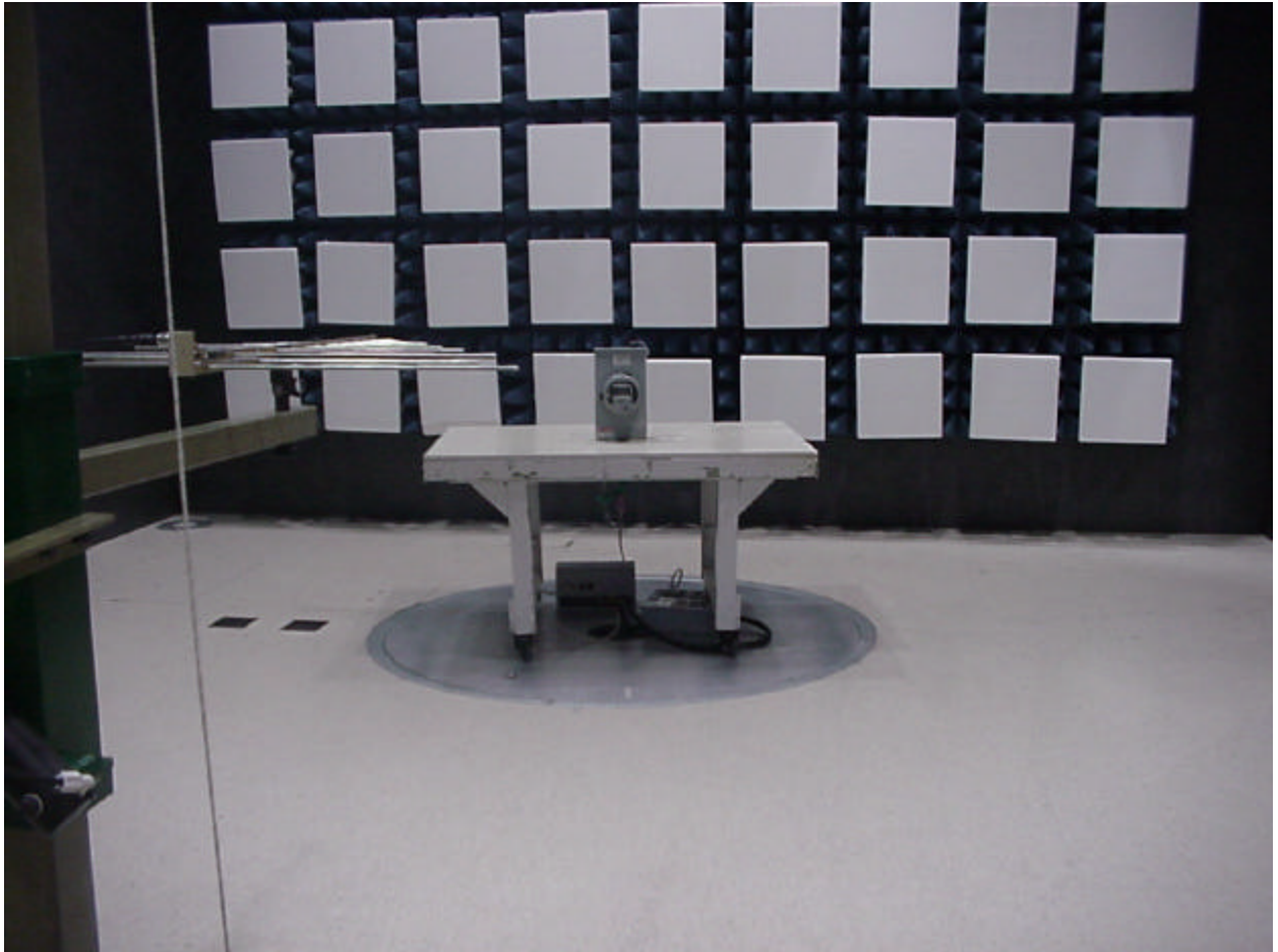
Figure 1 - Radiated Emissions Test Setup (Chamber – Front, X orientation)
