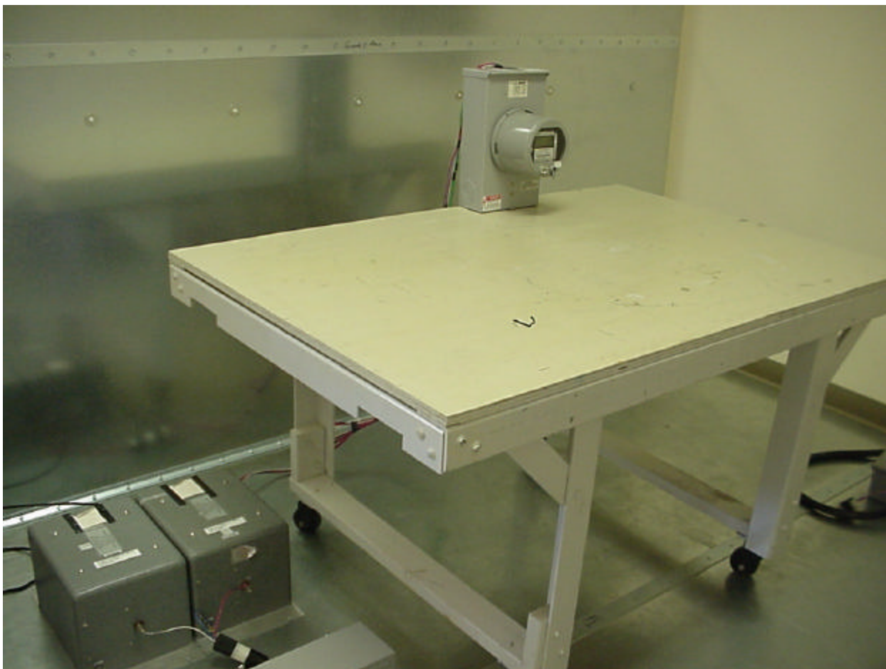
Figure 6 - Conducted Emissions Test Setup (Front)
