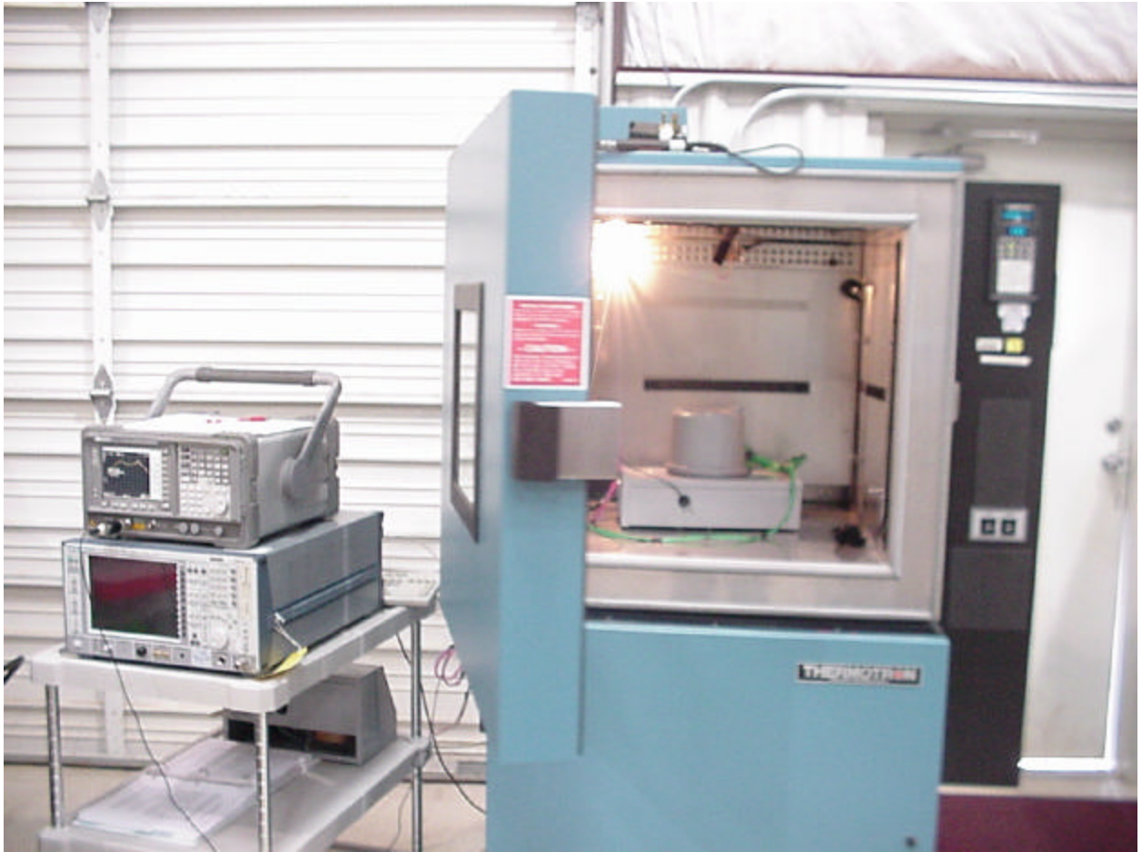
Figure 3 – Temperature Chamber Setup
