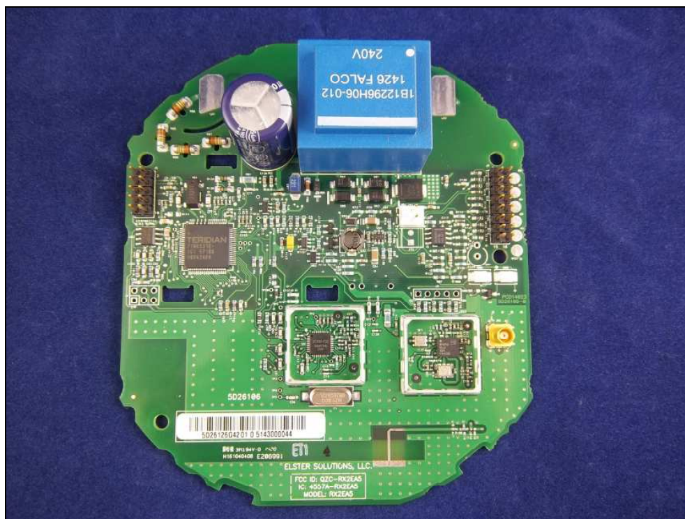
Figure 5: Internal Photo – Shields Removed
