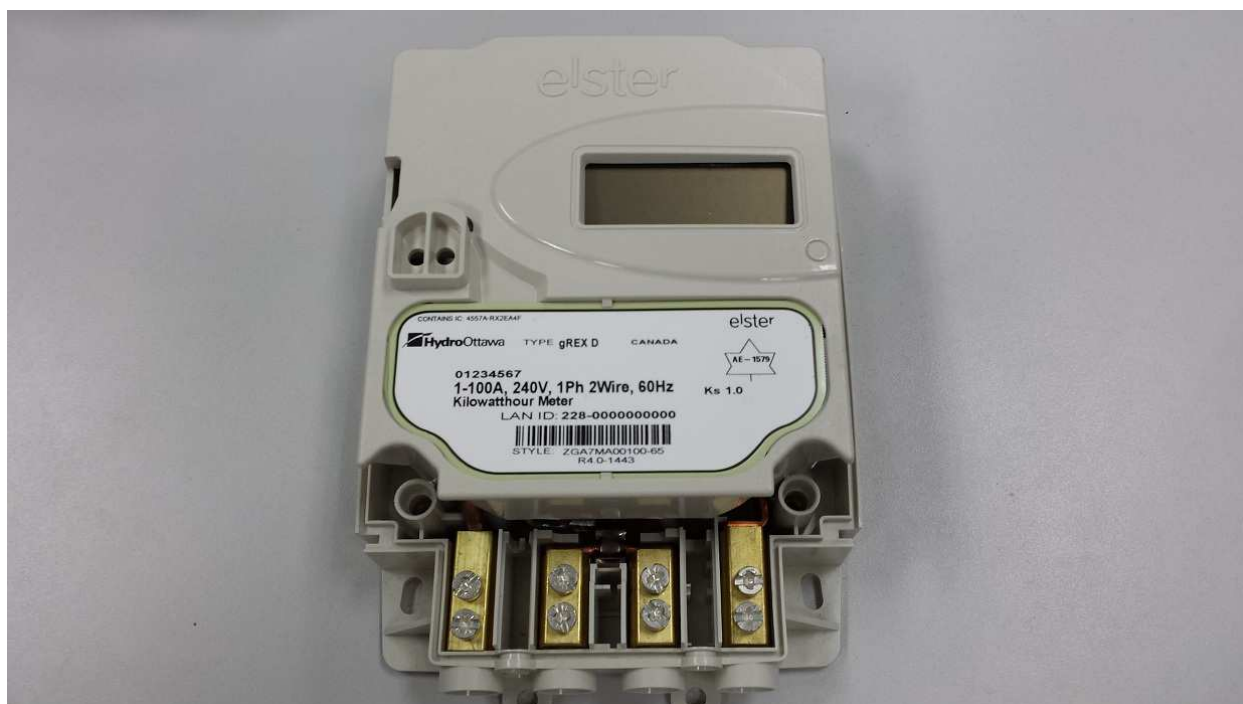
Figure 6: Host Label Location (gREX IC)
