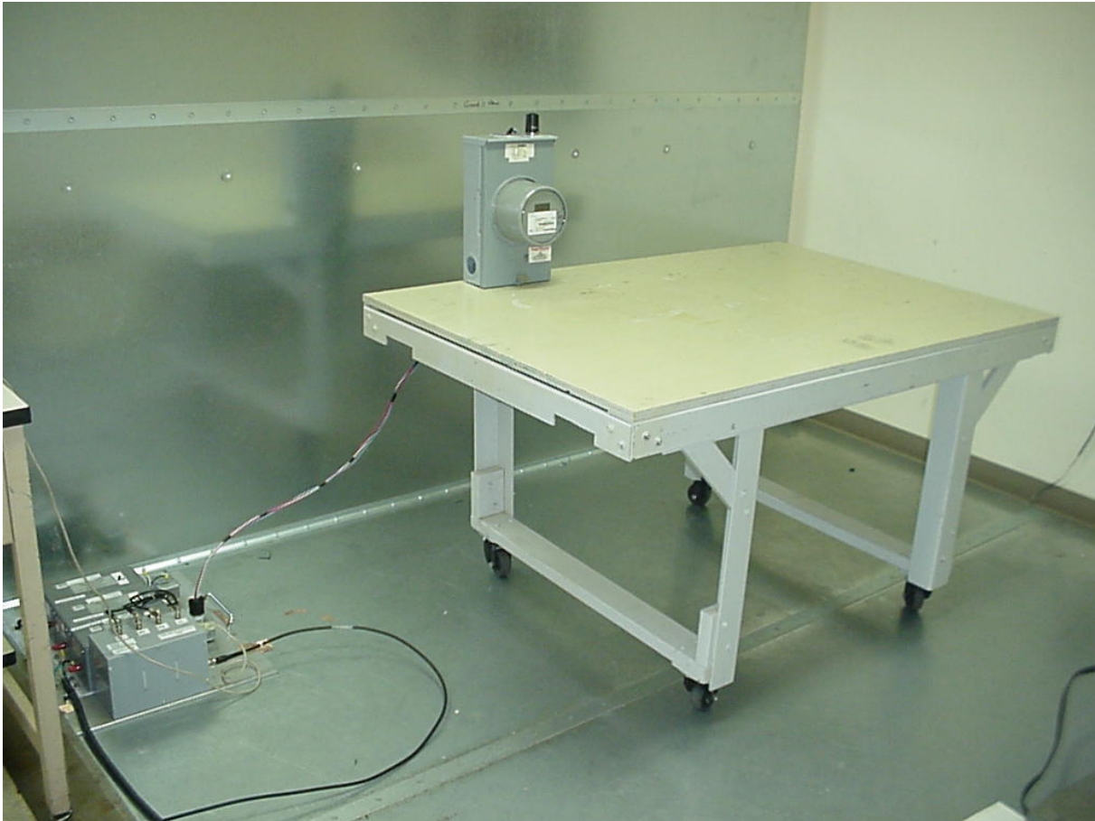
Figure 9 - Conducted Emissions Test Setup (Front)
