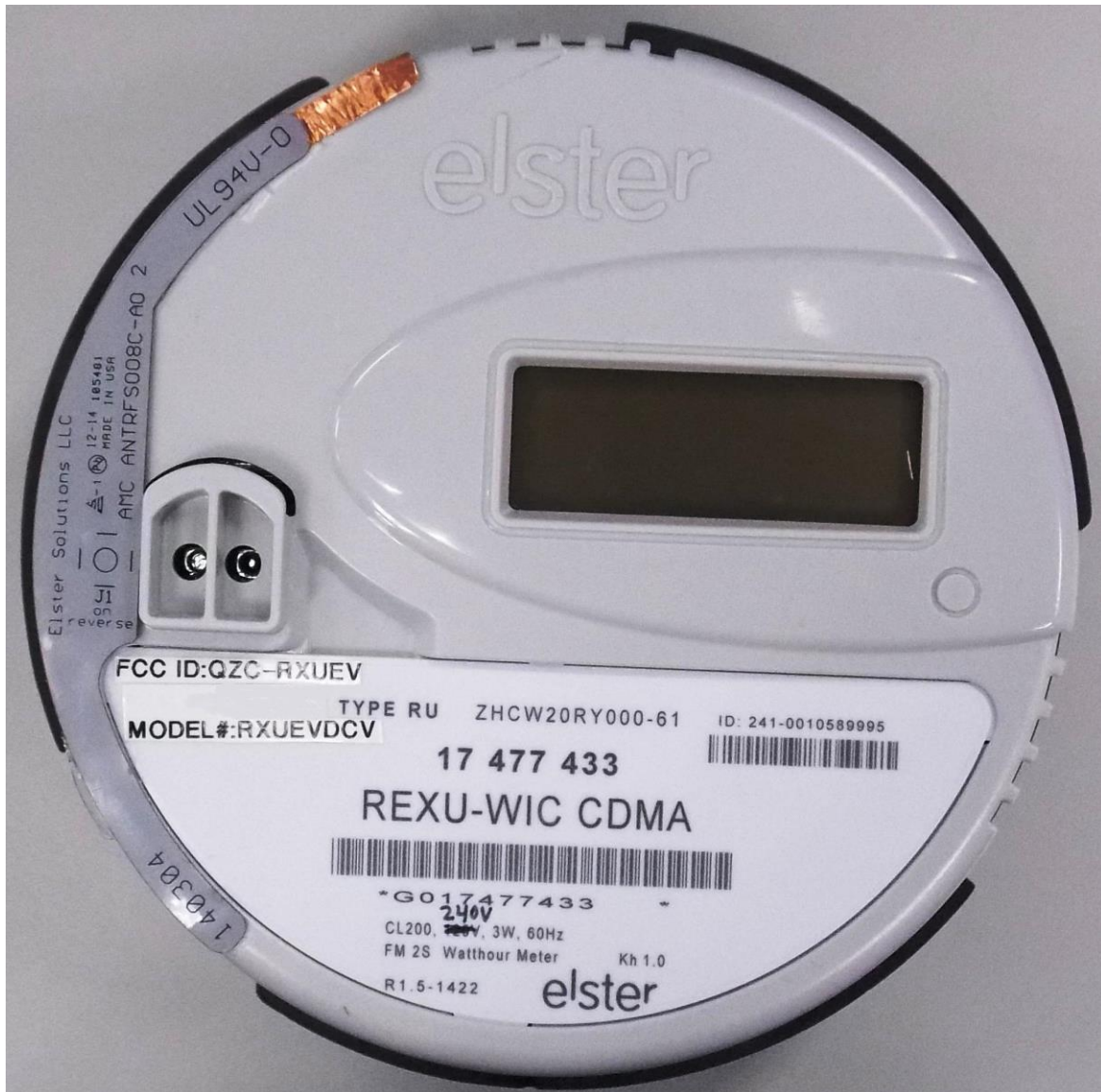
REXUniversal ® WWIC cellular antenna installed
