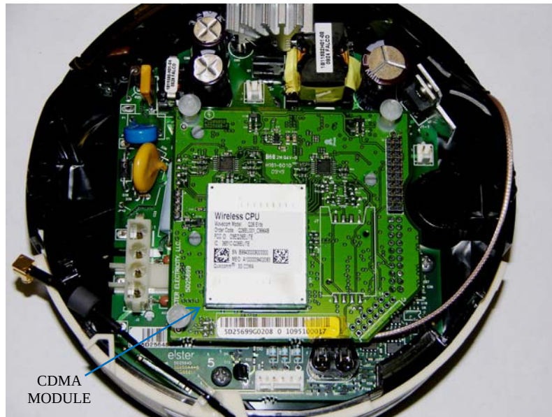
EA_Gatekeeper base module with WWIC PCB installed
