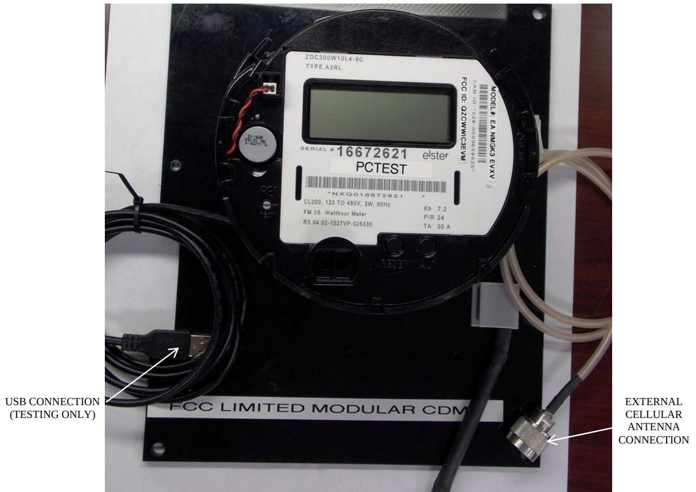
Modular EA_Gatekeeper complete module assembled to base
