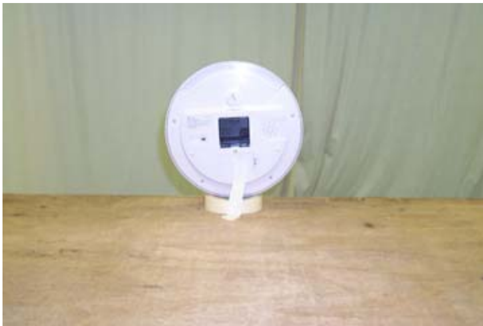
Figure 3.2 Radiated Test Setup Rear
