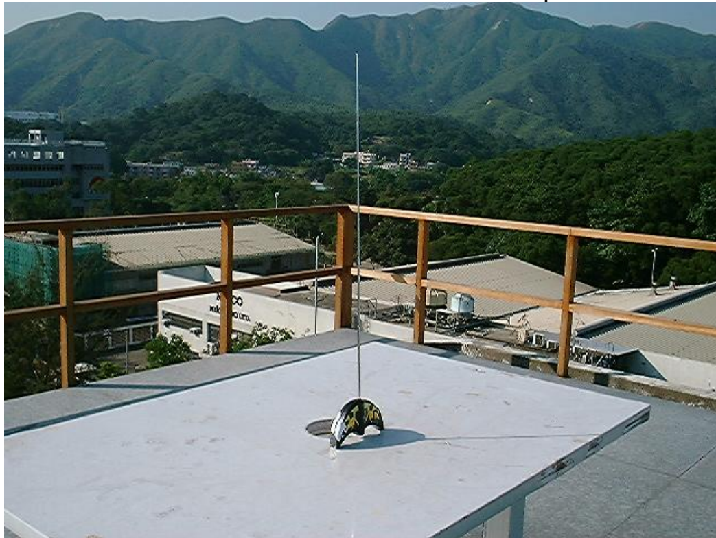
Measurement of Radiated Emission Test Set Up
