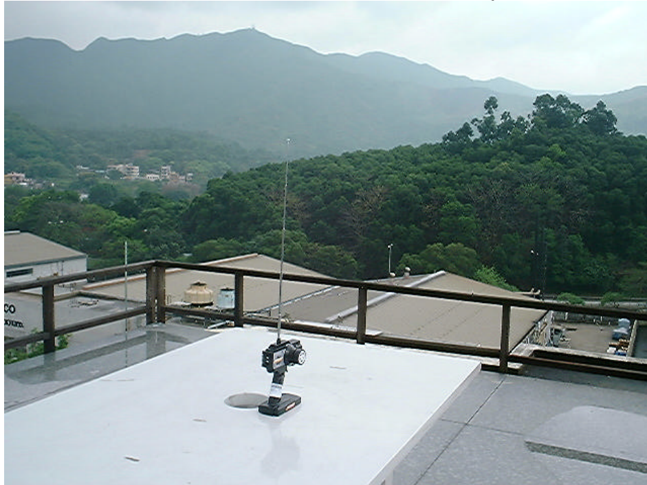
Measurement of Radiated Emission Test Set Up
