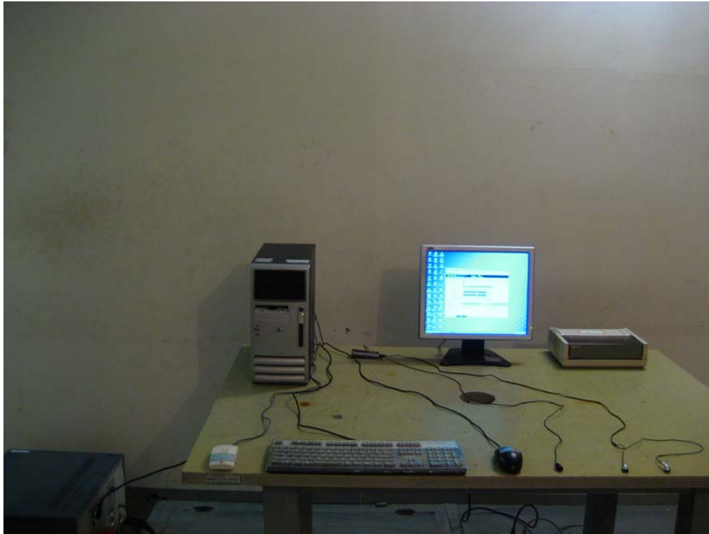
Conducted Emissions (PC power line) - Front View
