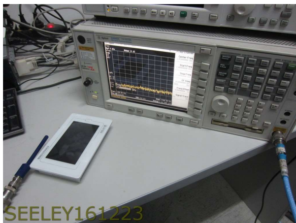
Frequency Hopping Tests – Wireless Smart Controller
