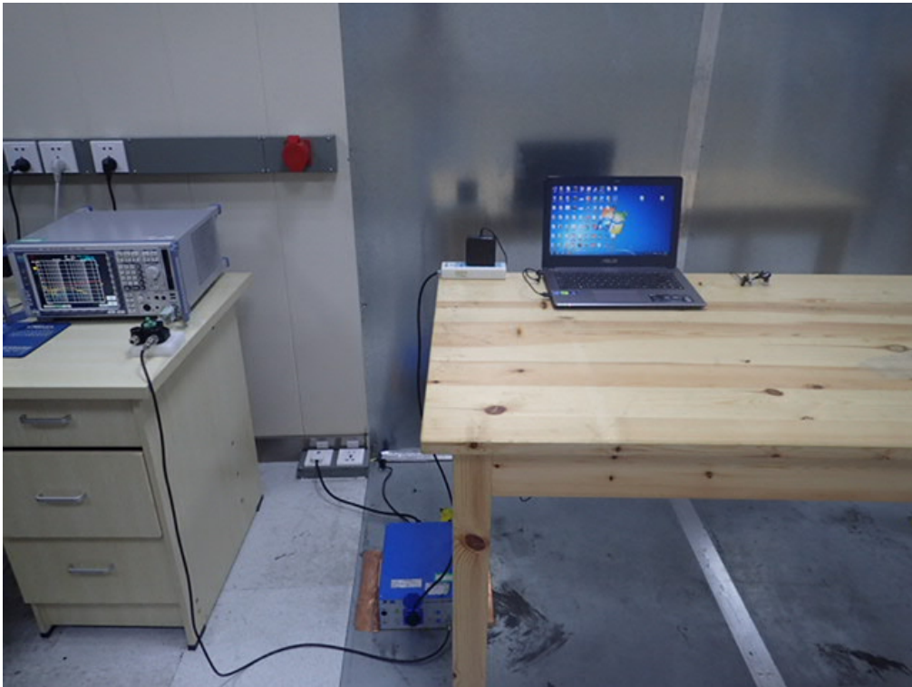
FCC RADIATED EMISSION TEST SETUP
