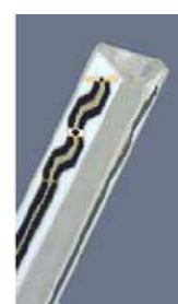
Figure 3.2 Probe Thick-Film Technique
