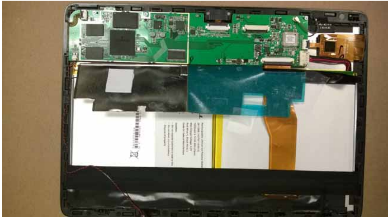
Photograph 9 – View of the PCB with the RF Shielding and ESD Tape Removed
