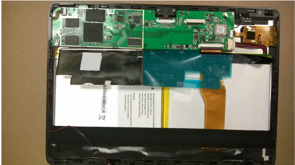
View of the PCB with the RF Shielding and ESD Tape Removed
