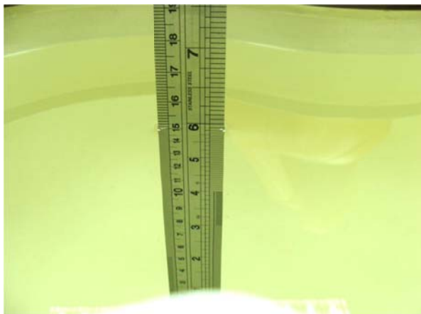
Fig 6.1 Photo of Liquid Height for Head SAR
