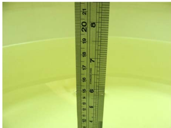
Fig 6.2 Photo of Liquid Height for Body SAR
