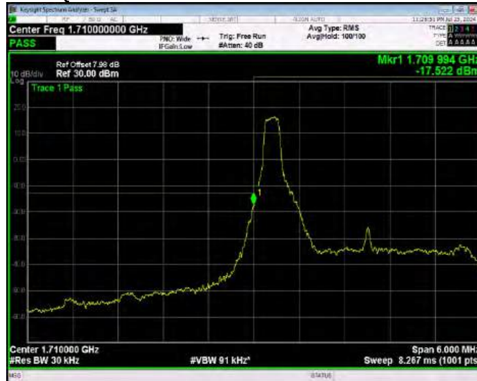
Band66 16QAM BW=3MHz Channel=131987 RB Size=1 Position=#Max Extended
