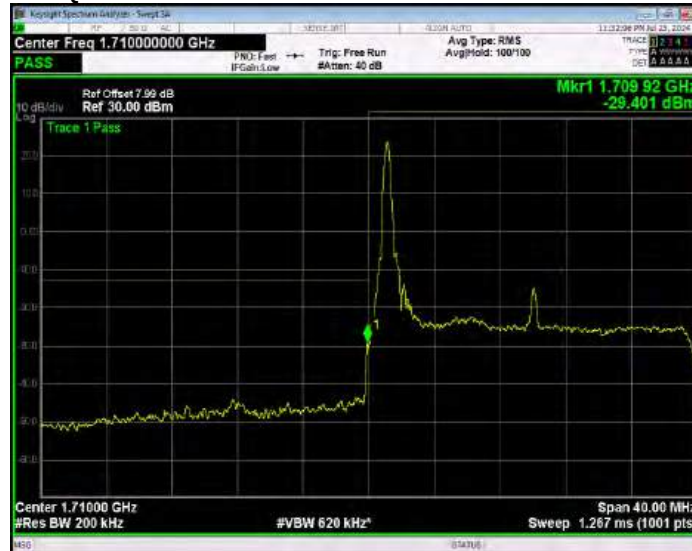
Band66 QPSK BW=20MHz Channel=132072 RB Size=1 Position=#Max Extended
