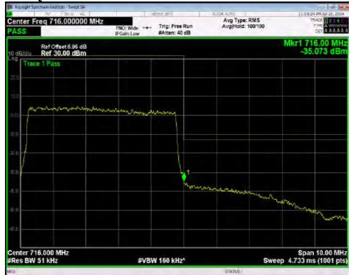
Band17 QPSK BW=5MHz Channel=23825 RB Size=25 Position=#0 Normal
