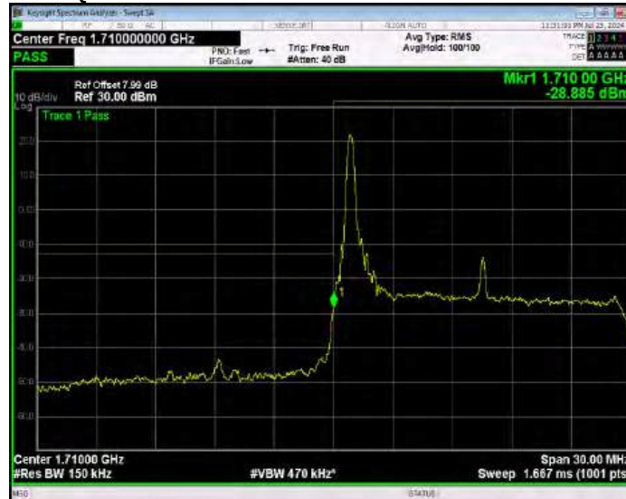
Band66 16QAM BW=15MHz Channel=132047 RB Size=1 Position=#Max Extended
