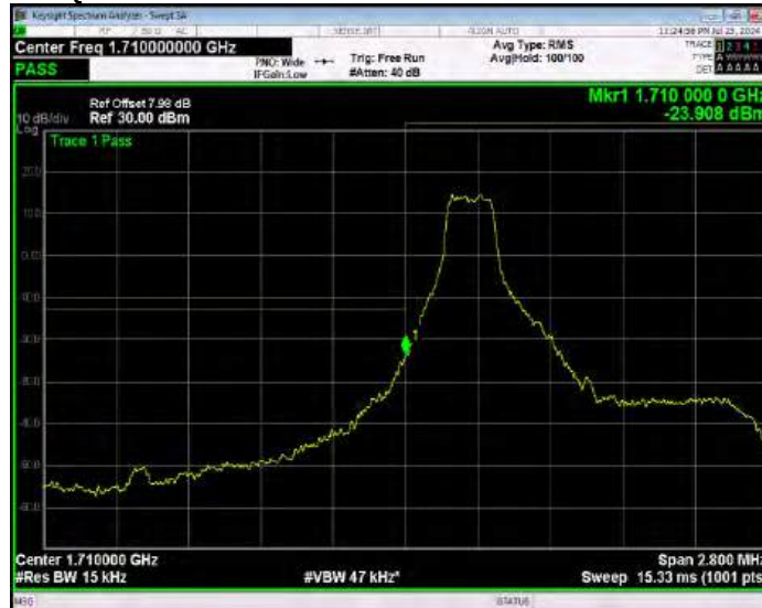
Band66 QPSK BW=1.4MHz Channel=131979 RB Size=1 Position=#Max Extended
