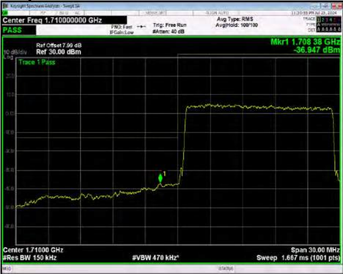
Band66 QPSK BW=15MHz Channel=132047 RB Size=75 Position=#0 Normal
