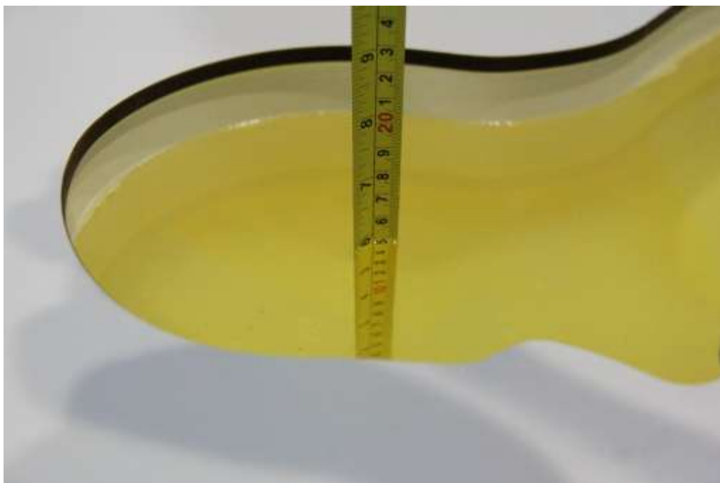
Picture 7-5: Liquid depth in the Head Phantom(2450MHz)
