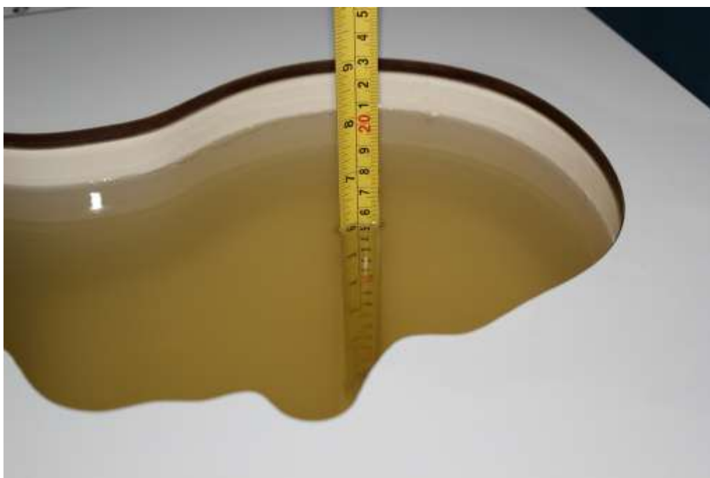
Picture 7-6: Liquid depth in the Head Phantom(2550MHz)
