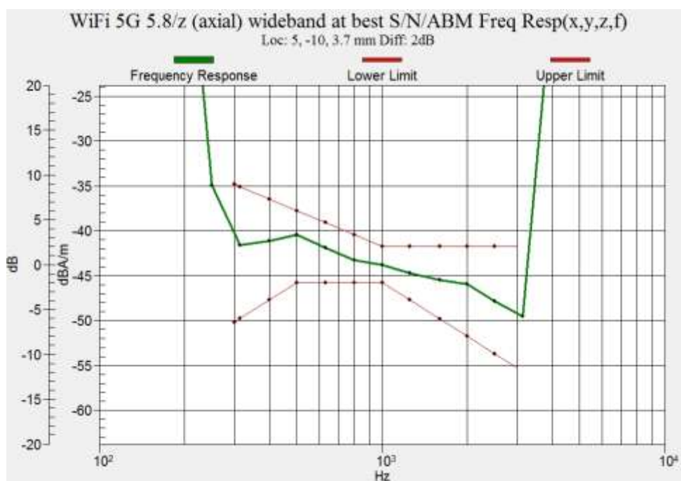
Figure B.24 Frequency Response of WIFI 5.8G
