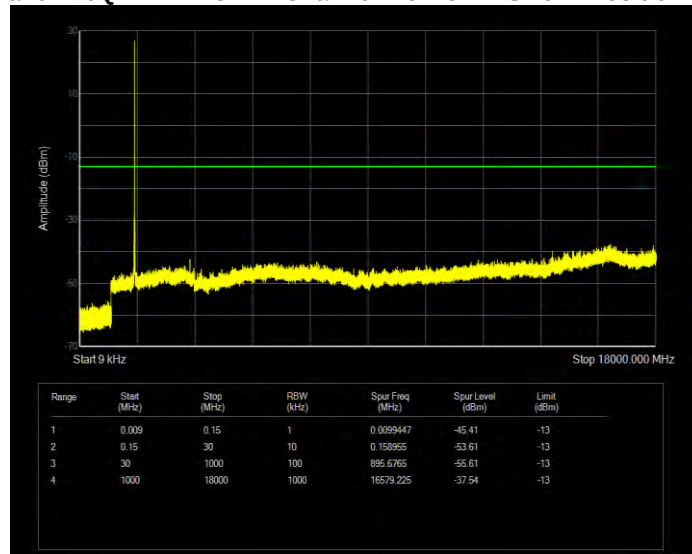
Band4 16QAM BW=5MHz Channel=20375 RB Size=1 Position=#0
