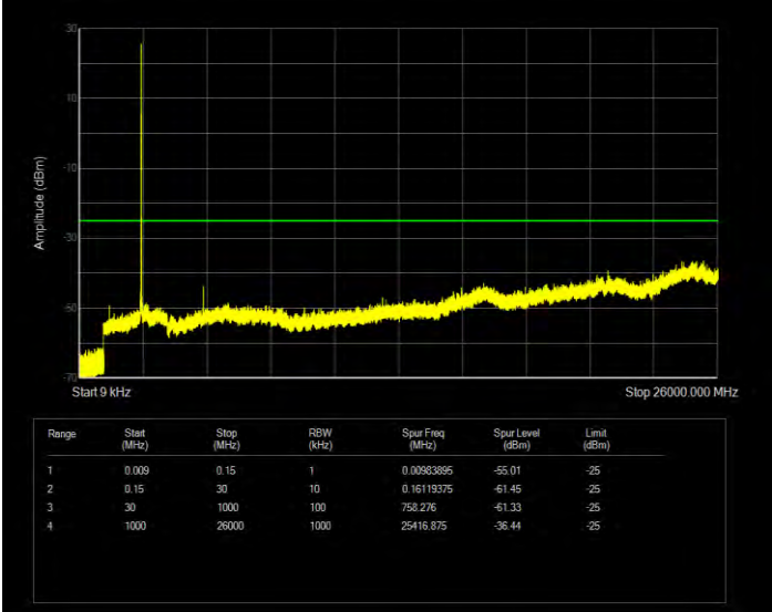
Band7 QPSK BW=5MHz Channel=21425 RB Size=1 Position=#0
