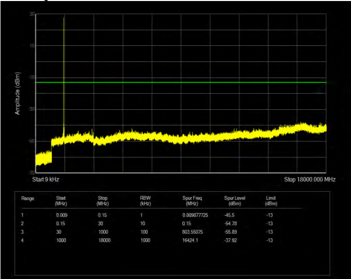
Band4 16QAM BW=1.4MHz Channel=20393 RB Size=1 Position=#0
