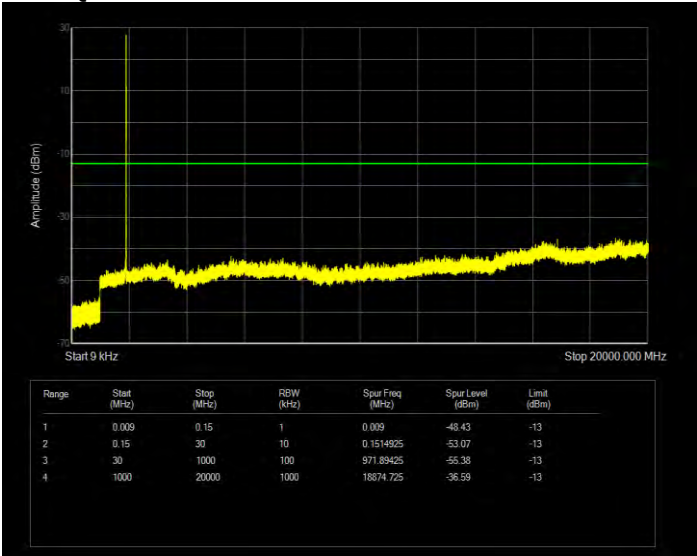
Band2 QPSK BW=3MHz Channel=19185 RB Size=1 Position=#0
