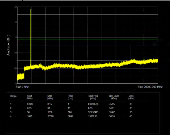
Band2 16QAM BW=1.4MHz Channel=19193 RB Size=1 Position=#0
