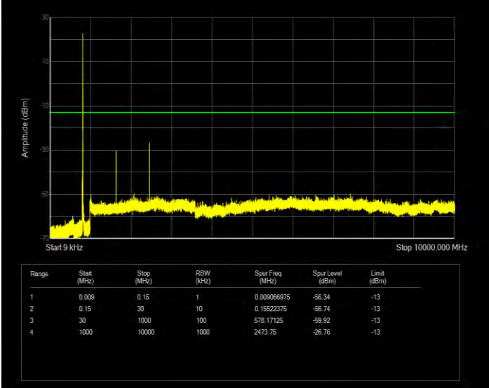
Band5 QPSK BW=5MHz Channel=20525 RB Size=1 Position=#0
