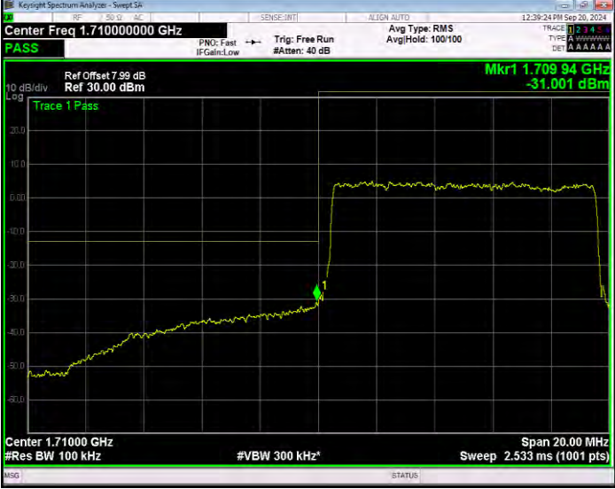
Band4 QPSK BW=10MHz Channel=20000 RB Size=50 Position=#0 Normal
