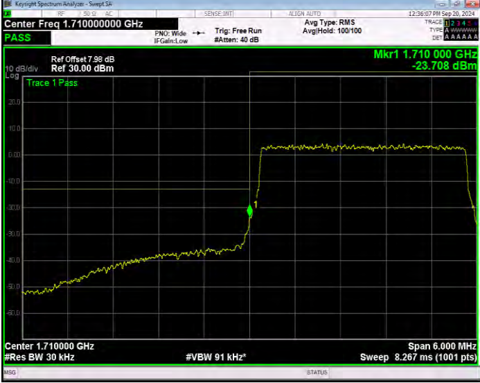
Band4 16QAM BW=3MHz Channel=19965 RB Size=15 Position=#0 Normal
