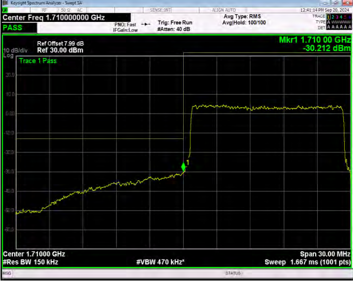
Band4 QPSK BW=15MHz Channel=20025 RB Size=75 Position=#0 Normal
