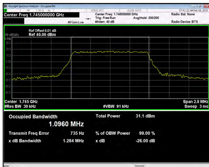
Band66 QPSK BW=1.4MHz Channel=132665 RB Size=6 Position=#0
