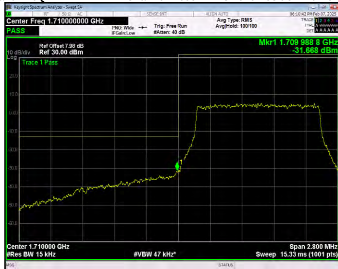
Band4 16QAM BW=1.4MHz Channel=20393 RB Size=1 Position=#0 Extended
