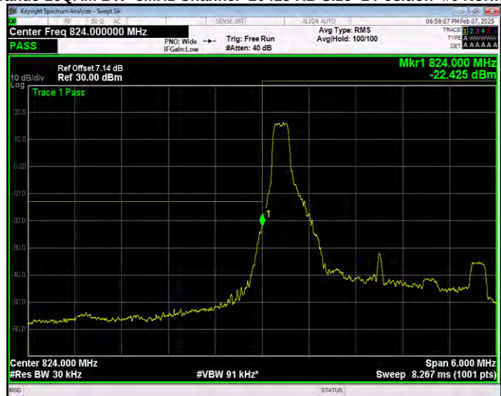
Band5 16QAM BW=3MHz Channel=20415 RB Size=1 Position=#Max Extended
