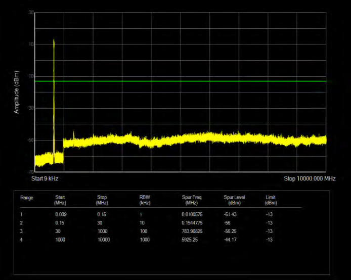
Band71 QPSK BW=10MHz Channel=133297 RB Size=50 Position=#0
