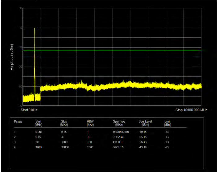
Band71 16QAM BW=15MHz Channel=133397 RB Size=75 Position=#0
