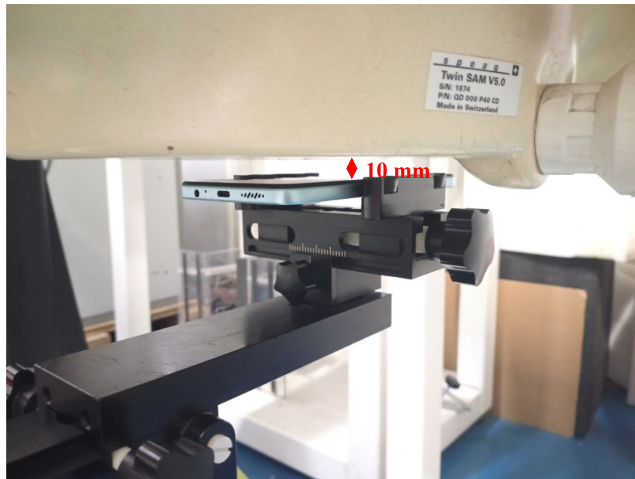
Body (Worn) Front Setup Photo(10mm)
