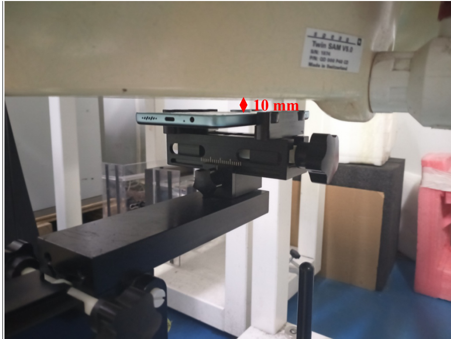
Body (Worn) Front Setup Photo(10mm)
