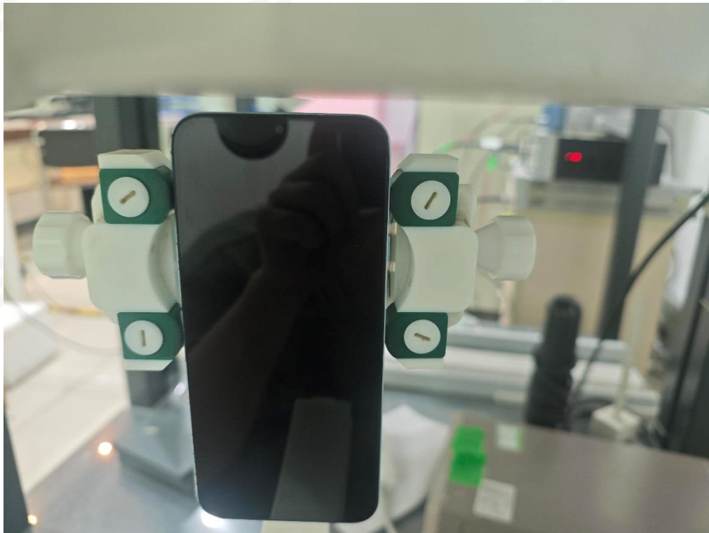
Body Top side(separation distance is 10mm)
