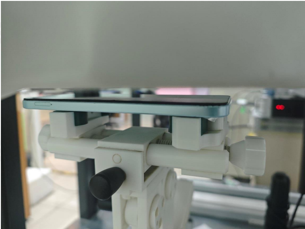
Body Front side(separation distance is 10mm)
