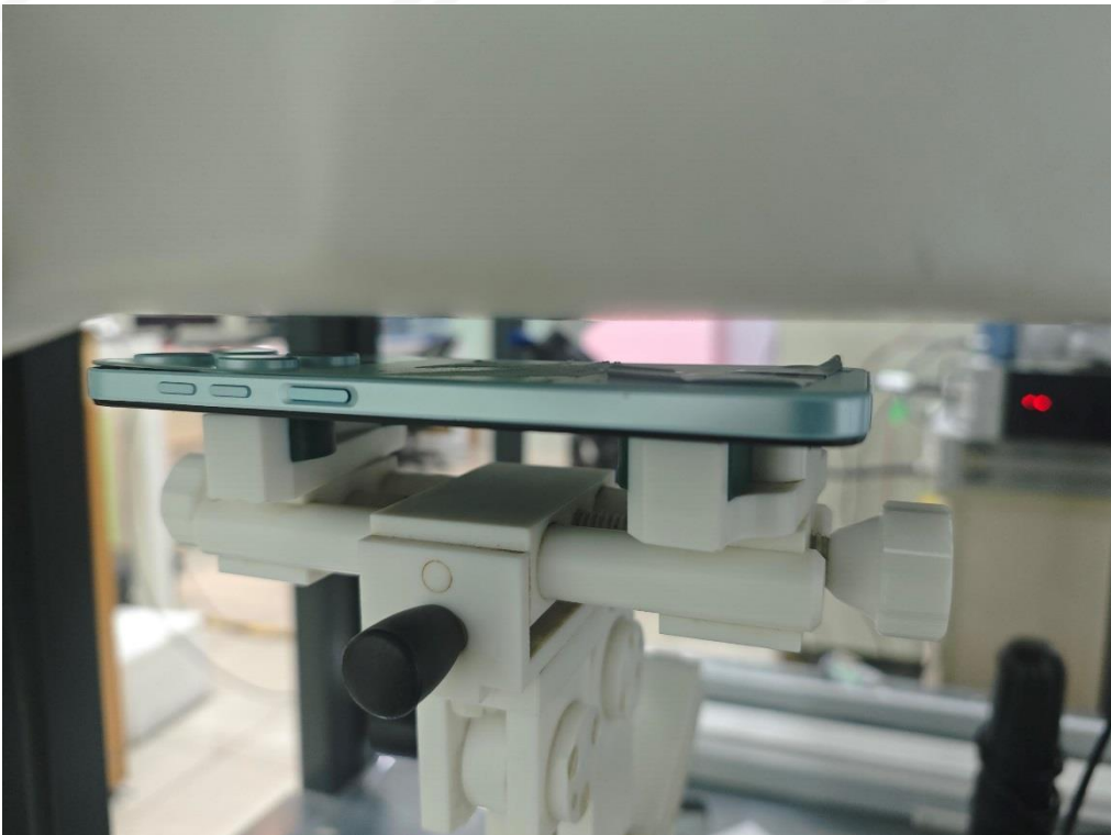
Body Back side(separation distance is 10mm)
