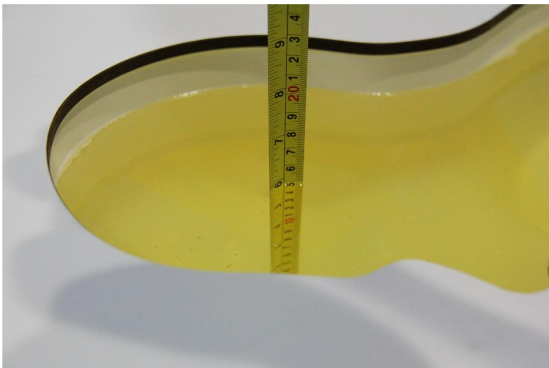
Picture 7-9: Liquid depth in the Head Phantom(2450MHz)
