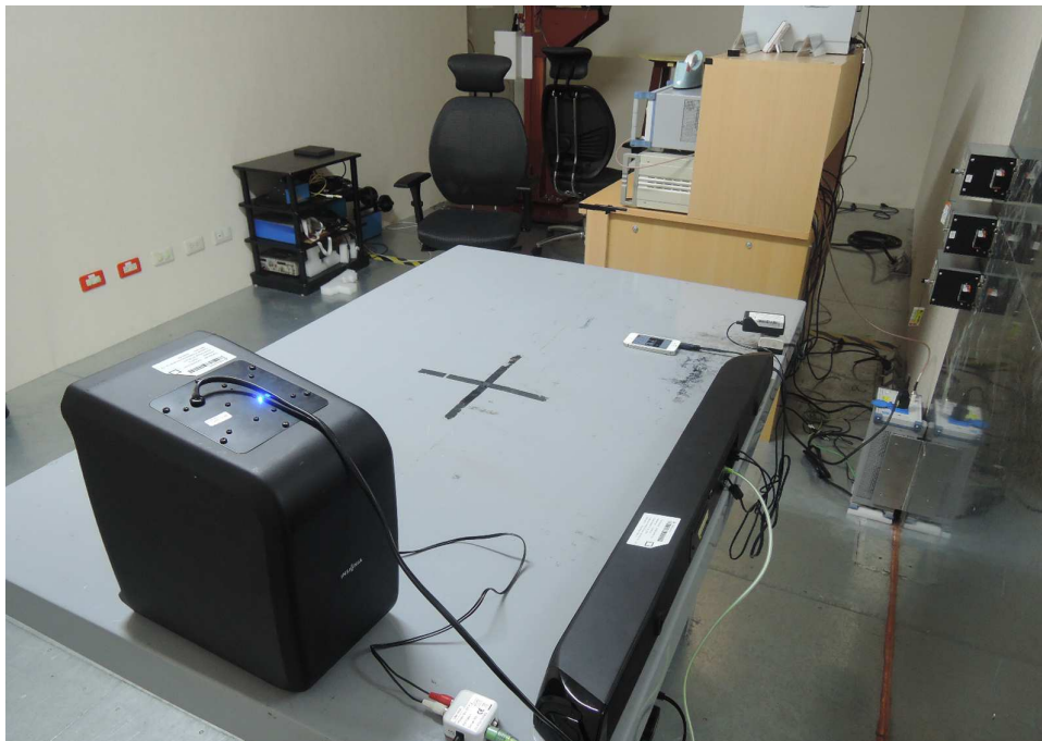
Photograph 5: Set-up for for Mains Conducted testing Back
