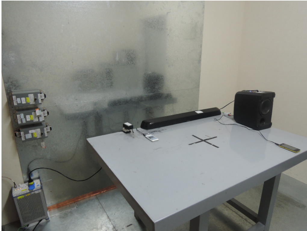
Photograph 6: Set-up for for Mains Conducted testing Front
